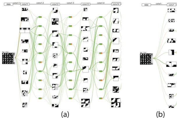
Figure 4. The comparison between LeNet and DeepLeNet: (a) the weights of the first group of convolutional layers in DeepLeNet; (b) the weights of the first convolutional layer in LeNet.
