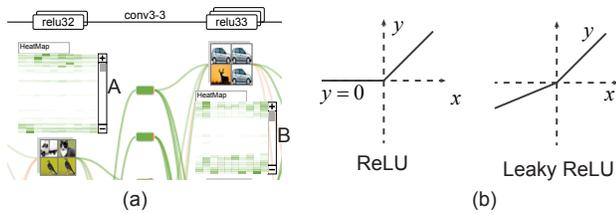
Figure 7. Illustration of activations: (a) the neurons with zero activations in layers relu3-2 and relu3-3 (output of corresponding convolutional layers); (b) illustration of ReLU and leaky ReLU.
