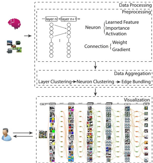
Figure 2. CNNVis system pipeline.
